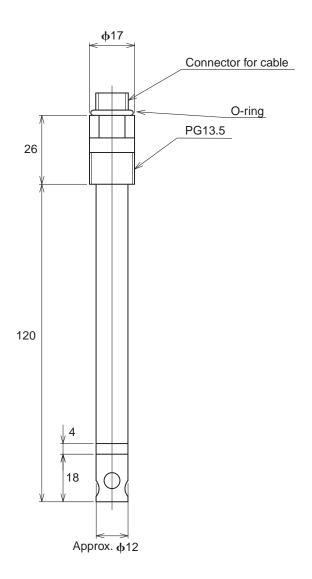
Unless otherwise specified, differences in the dimensions are specified as: General tolerance=(Criteria of tolerance class IT18 in JIS B0401-1986)/2.
